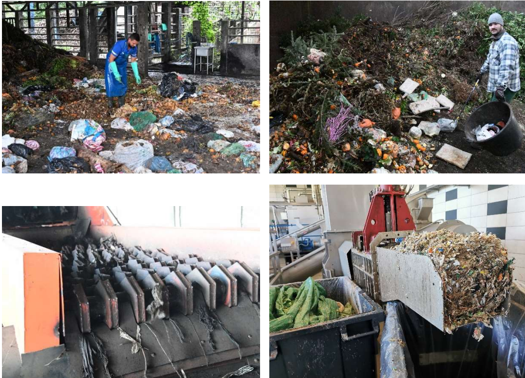
Examples of infrastructure for sorting delivery scales. Manual sorting on the ground (top), sieve for coarse plastics removal (bottom left), hammer mill (bottom right).
