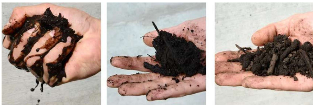
Fist test to determine the water content of compost Left: compost too moist. Center: compost with optimum moisture content. Right: compost too dry.
