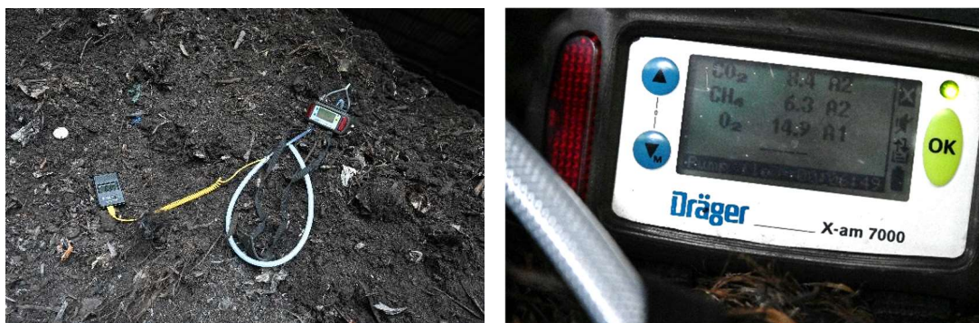
Measuring gas composition in a windrow.
