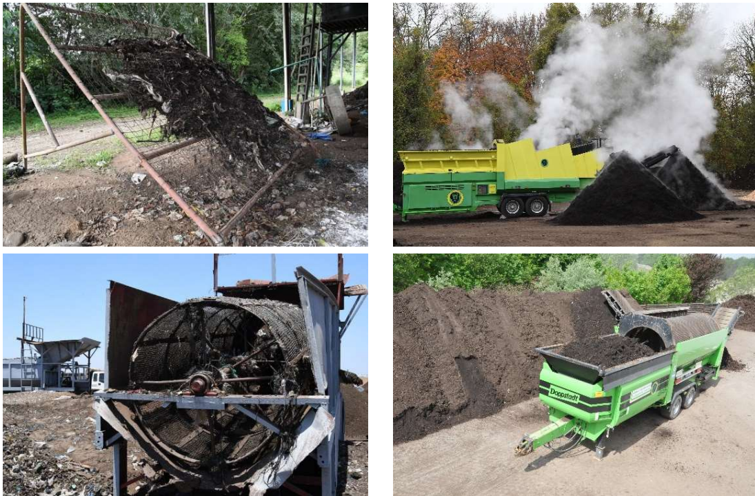
Examples of screening machines: handmade sieves (top left), star sieves (top right) and rotary drum sieves (bottom).
