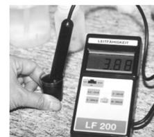
$$\text{Salzgehalt (in KCl}_{\text{eq}}/\text{kg TS)} = \text{EC (in mS/cm)}/\text{TS (in \% FS)} \times 583,4$$
