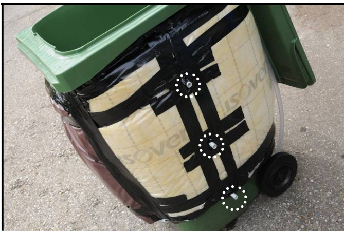
Test composter: view of holes for temperature and gas measurements
