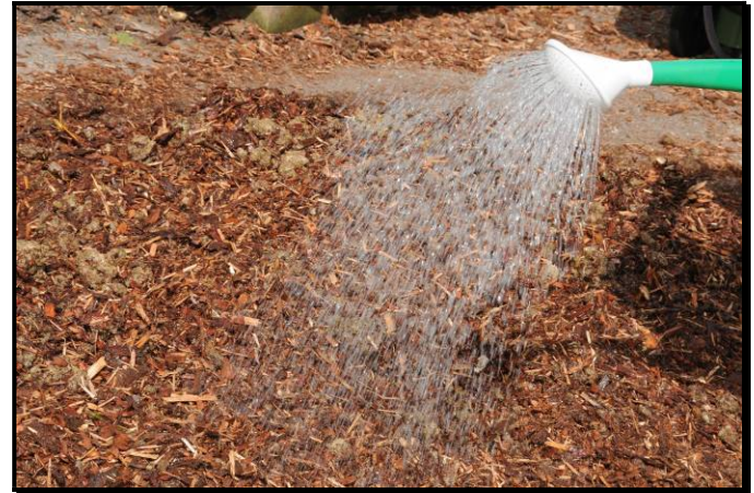
Preparation of mixture to test: add water to mixture until optimal moisture
