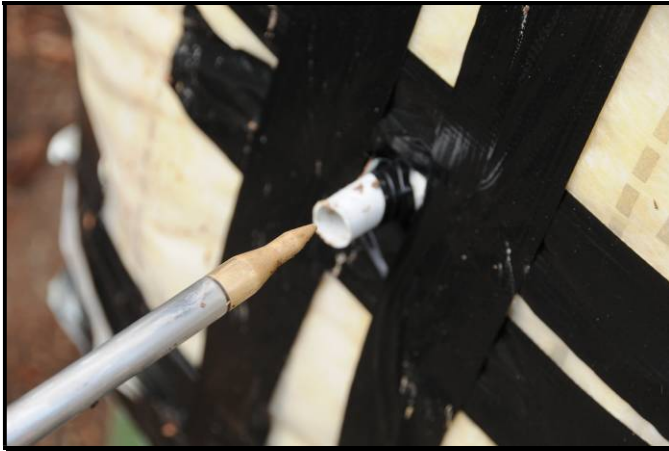
Measurement of temperature (at the different heights of the composter)
