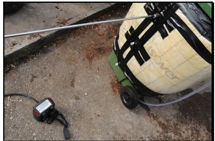
Measurement of gas composition (at the different heights of the composter)
