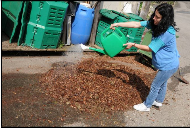
Preparation of mixture to test: add water to mixture until optimal moisture
