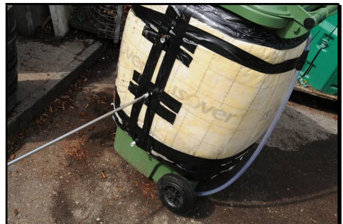
Measurement of temperature (at the different heights of the composter)
