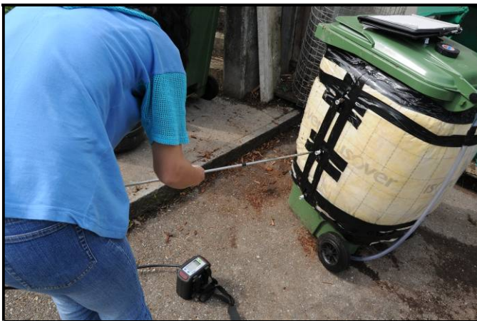
Measurement of gas composition (at the different heights of the composter)
