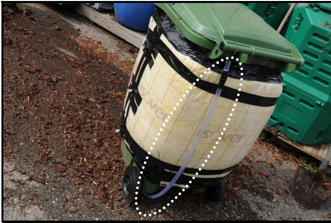
Test composter: view of the flexible pipe for the evacuation of leaching juices 240 liter
