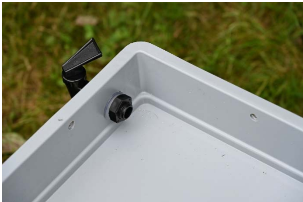
Fig. 1. View of the tap installed on the system's lower tray and the ventilation holes.
