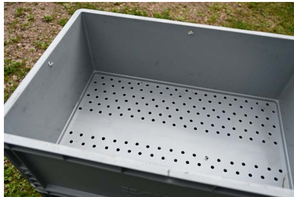
Fig. 2. View of the bottom of the trays with numerous 8.5 mm diameter holes, and ventilation holes at the top of the sides of the trays.
